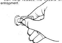
To lock or unlock the freezer you must hold the key in the lock while turning. The lock is spring loaded so the key cannot be left in the lock.
